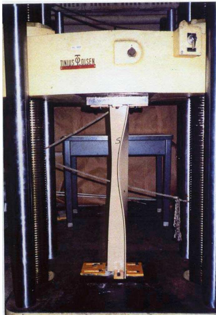
Full section column testing was conducted on Bedford Reinforced Plastics' Equal Leg Angles, I-Beams, H-Beams, and Square Tubes.
